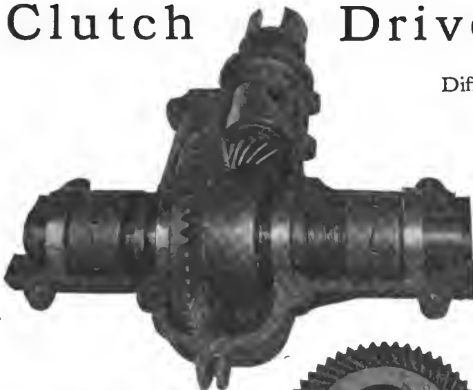
Allen compensating axle and its principal component parts
